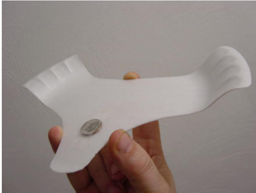
If the glider stalls or "porpoises", this means the weight is a bit too far back and should be moved forward. Should the glider nose dive, it means that the weight is too far forward and should be moved back. After a few flights, you should have the weight positioned correctly, so burnish the tape down to securely hold the weight.
